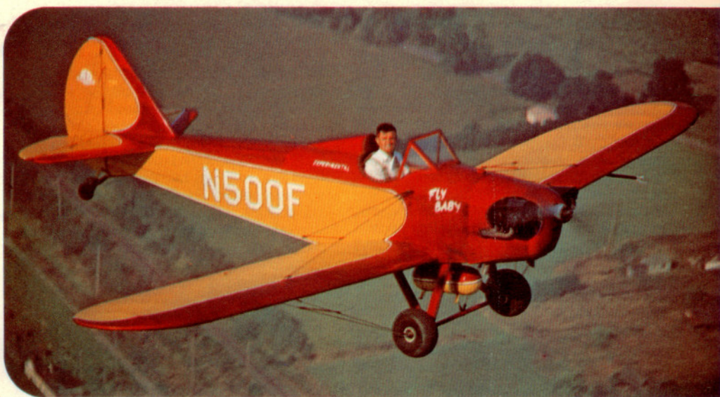
Although a "Latter-Day Antique" in appearance and construction, all-wood Bowers "Fly Baby" won EAA Design Contest for easy-to-build, easy-to-fly beginner's homebuilt. Does well on 65–85 h.p.; larger engines introduce structural and weight penalties.
