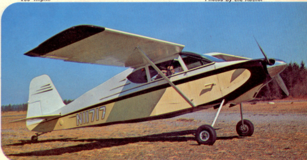
Nesmeth "Cougar," patterned after Steve Wittman's "Tailwind," combines with it to be the most popular of the homebuilt two-seaters. Power from 85 to 125 h.p. gives this 21-foot span wood and tube side-by-side design a cruising speed up to 160 m.p.h. Photos by the Author
