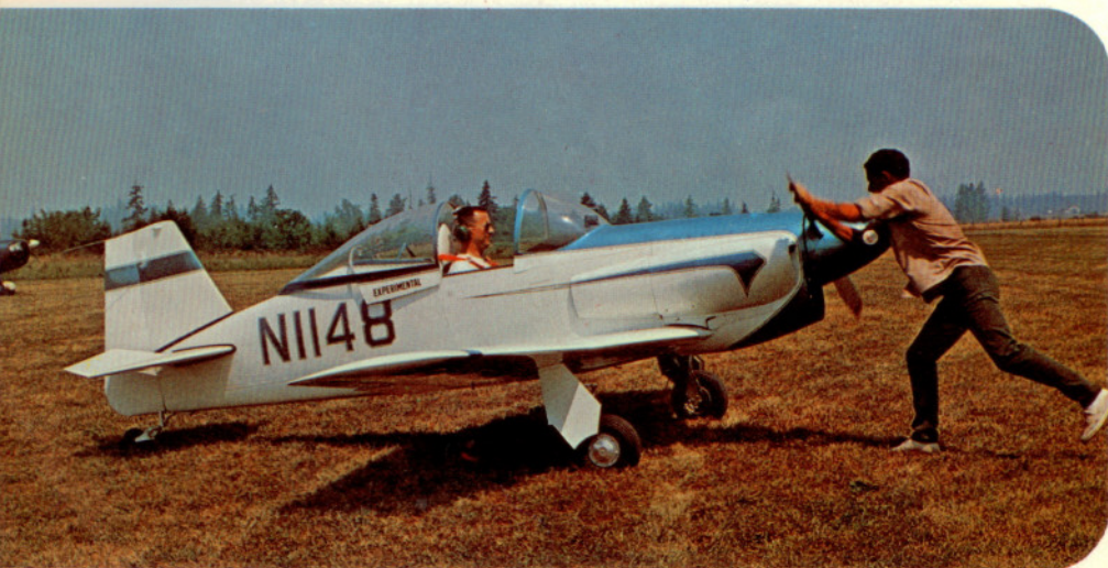
All-metal Long "Midget Mustang" was designed in 1947 to be a production article for sport or racing. Plans now on the market for homebuilders. This modified version has 18½ foot span and retractable gear; cruises 160 m.p.h. on 108 h.p. Starting is by hand.
