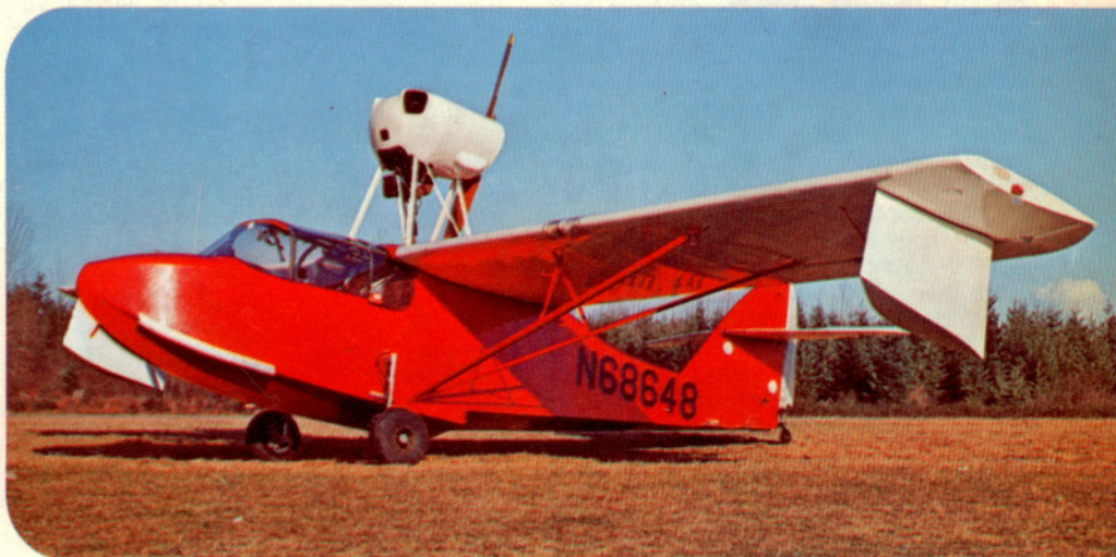
Volmer VJ-22 "Sportsman" features a wooden hull and 100 h.p. engine installation that can use wing and tail surfaces from Aeronca "Chief/Champion," Taylorcraft, or Piper "Cub." FAA permits use of factory-built parts on homebuilts within reasonable limits.
