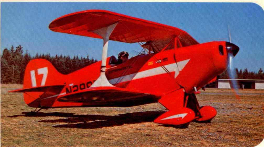
Pitts biplane was first used by air show aerobatic pilots in late 1940's, now is popular with the homebuilders. Most use 85-125 h.p.; some show types carry 180. This 125 h.p. version was 1966 champion in new racing class for open cockpit sport biplanes.
