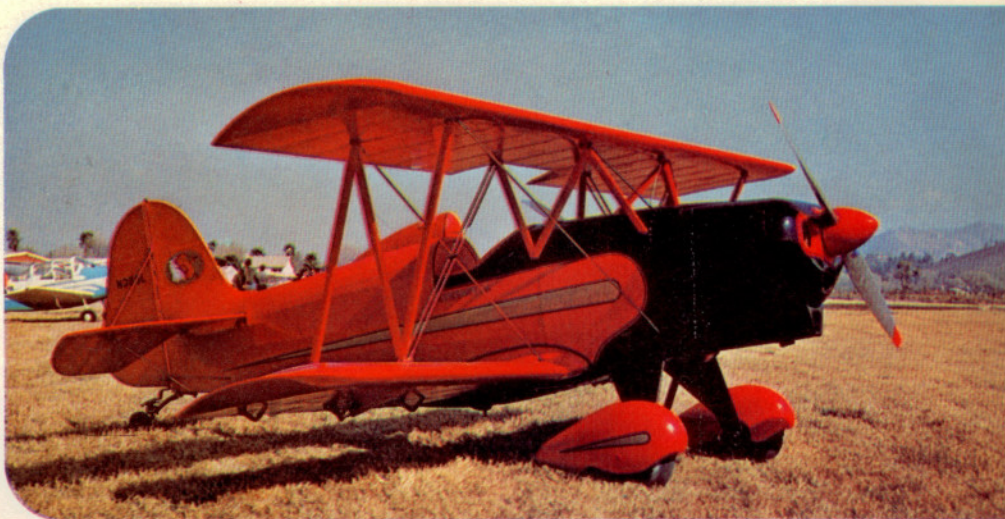
Smith DSA-1 "Miniplane" is most popular of the homebuilt biplanes. Original 65 h.p. produced marginal performance so majority have moved into the 85-125 h.p. range. With adequate power, such a midget can do recreational and even good air show aerobatics.
