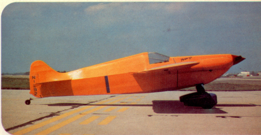
Wittman "Bonzo" was near-duplicate of 1947 Goodyear Racer "Buster," itself rebuilt from a prewar racer. With 85 h.p. engines over-revved to 3600 r.p.m. these 14-to-16-foot span midgets can do over 200 m.p.h. on the straightaways, but land over 80.
