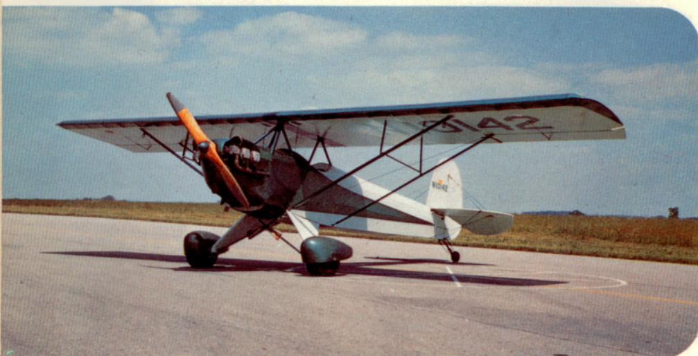
The Corben "Baby Ace" of the early 1930's was modernized for homebuilders by EAA's president Paul Poberezny in 1954. Fuselage and tail are welded steel tube, 25-foot wings are of wood. Most of these are flown with 65 h.p. engines, use some "Cub" parts.
