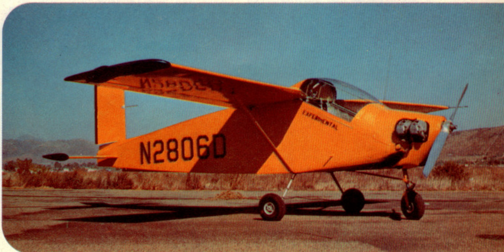
All-metal Andreasson BA-7, built while designer was employed by Convair, is now a production article; built by Malmo in Sweden and Bolkow in Germany. Some of the Bolkow "Juniors" have been imported into the United States and fitted with 100 h.p. Continental engines.
